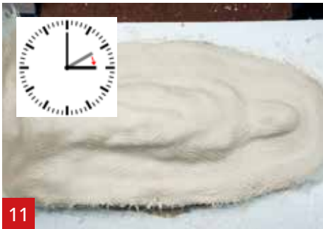
11 Let the A1 support mould dry for 60 minutes.
