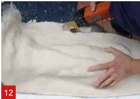
12 If desired, the A1 support mould can be finished with a multitool.
