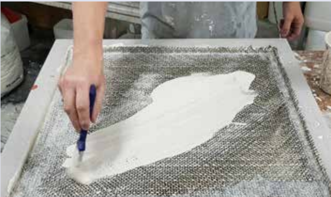
To laminate, you have to work wet in wet. A quick way to apply A1 is with a brush or roller.
