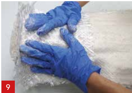
9 Press the A1 Triaxial fibre. The fibre can be formed/shaped well.
